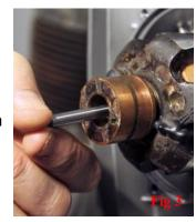
Step 2. Carefully assemble the two rings onto the stator with the cables exiting as shown. Ensure correct seating of the rings on the stator, if necessary gently tap them on with each ring so the 3 holes align with the 3 slots in the stator to allow the screws to pass through, see Fig 5 & 6.
