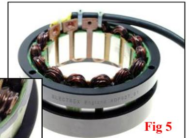
Step 2. Carefully assemble the two rings onto the stator with the cables exiting as shown. Ensure correct seating of the rings on the stator, if necessary gently tap them on with each ring so the 3 holes align with the 3 slots in the stator to allow the screws to pass through, see Fig 5 & 6.
