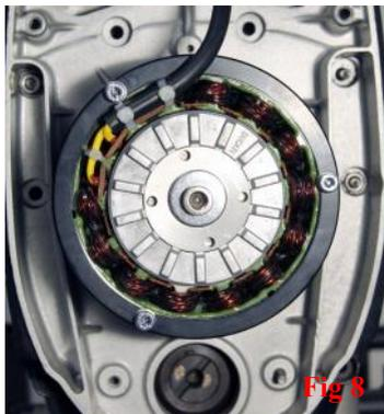
Step 4. Fit the rotor onto the shaft using the original bolt and large washers provided see Fig 8. Tighten bolt to specified torque. Check the rotor is not touching the stator, there must be a small air gap of approx. 0.5mm between the rotor and stator, this can be checked by inserting a slip of paper.
