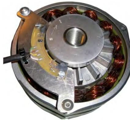
Figure 4 Connecting the pickup.
