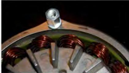
Figure 1 Threaded rods with spacer.
