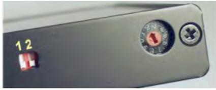
Figure 9 DIP switches and rotary switch.
